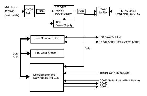
Figure 1-5: TPU Block Diagram
