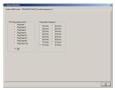
**Figure 4-95:** The Sonar Interface Dialog Box, Series 3000 Sonar System—Responder Control Tab
