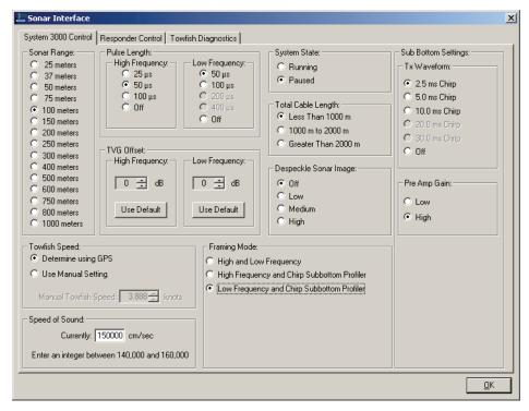
Figure 4-94: The Sonar Interface Dialog Box, Series 3000 Sonar System—System 3000 Control Tab
