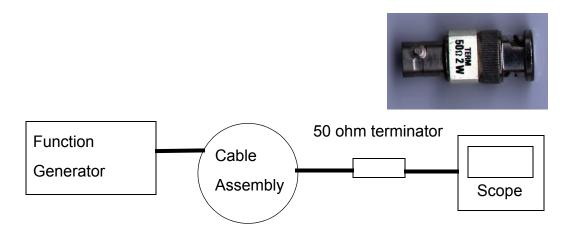
**Figure C-4:** Setup for Measuring Tow Cable Characteristics using a Function Generator, Terminator and Oscilloscope
