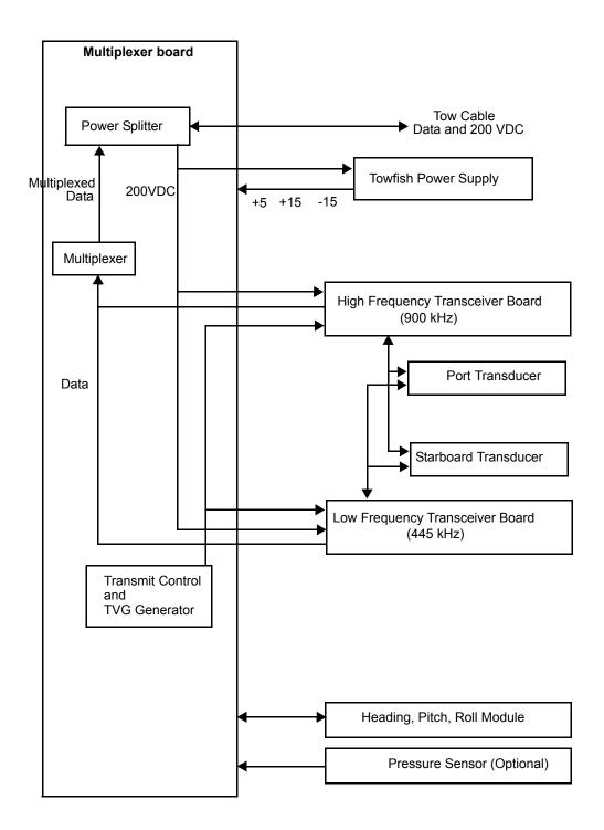
Figure 1-3: Towfish Block Diagram
