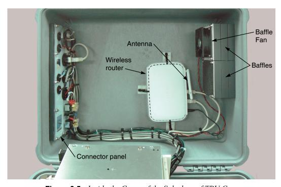
Figure 6-5: Inside the Cover of the Splashproof TPU Case
