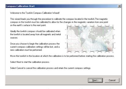
Figure 4-18: The Compass Calibration Wizard
