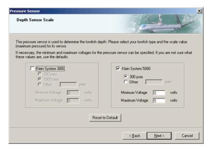
Figure 4-14: The Survey Wizard—Depth Sensor Scale Page
