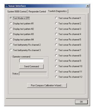
Figure 4-17: The Sonar Interface Dialog Box, Series 5000 Sonar System—Towfish Diagnostics Tab
