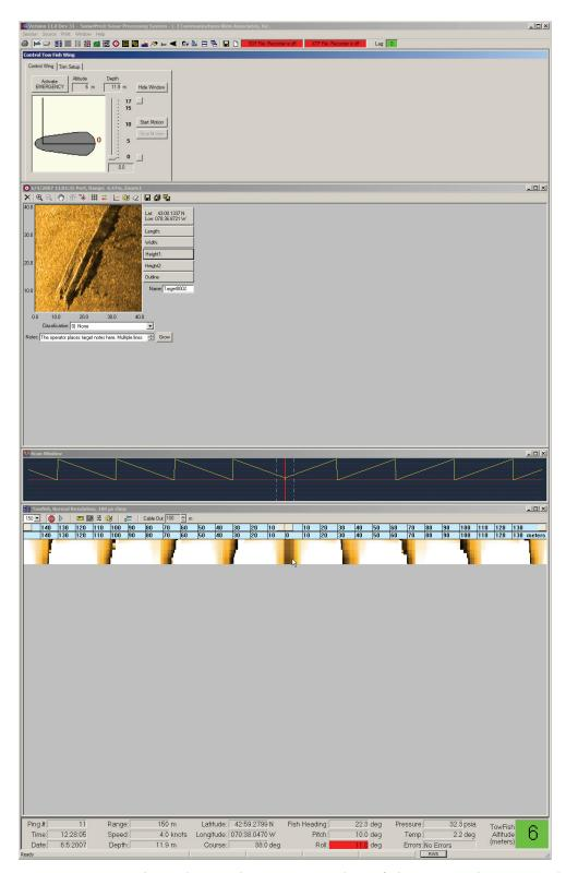
**Figure 4-77:** Dual Displays with Open Control Towfish Wing Dialog Box and Target Window (Top) and Sonar Viewer, Information and Scan Windows (Bottom)
