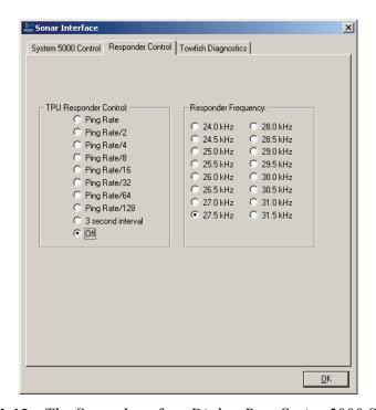
**Figure 4-16:** The Sonar Interface Dialog Box, Series 5000 Sonar System—Responder Control Tab
