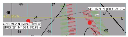
**Figure 4-41:** Position, Bearing and Distance Display Example in the Navigation Window
