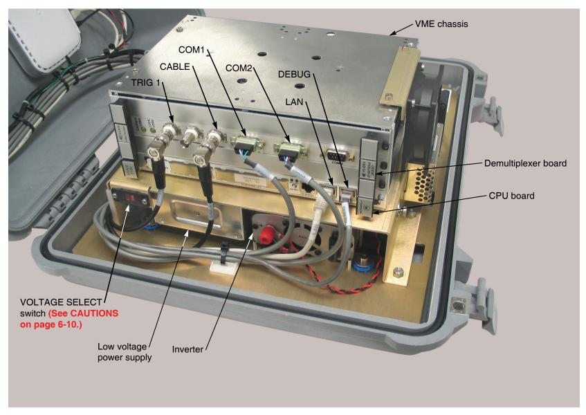
**Figure 6-6:** Front Panel of VME Chassis inside Splashproof TPU
