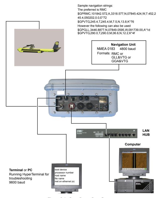
Figure C-1: Basic System Setup Diagram
