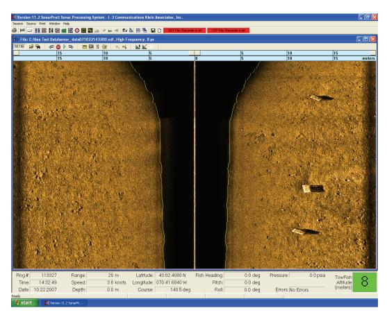
**Figure 4-97:** Sonar Viewer Window—900-kHz Operation with the Series 3900 Sonar System
