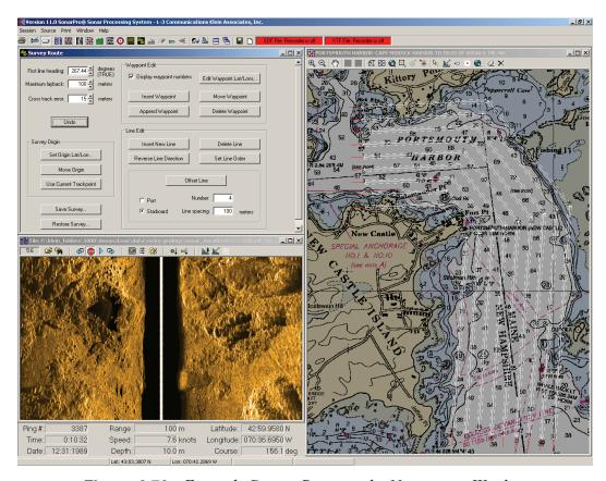
**Figure 4-70:** *Example Survey Route in the Navigation Window*
