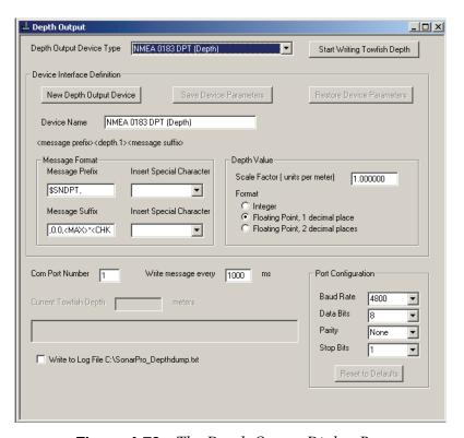
**Figure 4-73:** *The Depth Output Dialog Box*
