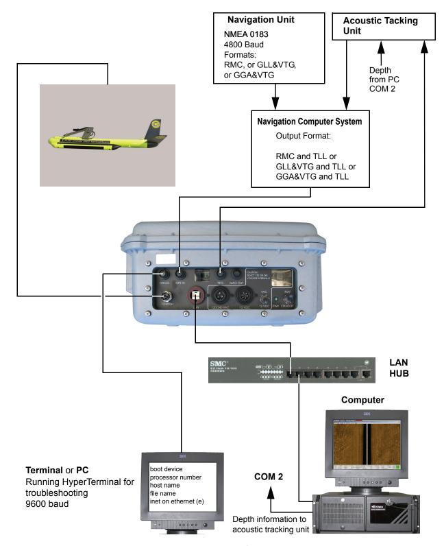
Figure C-2: System Setup Diagram with Acoustic Positioning System
