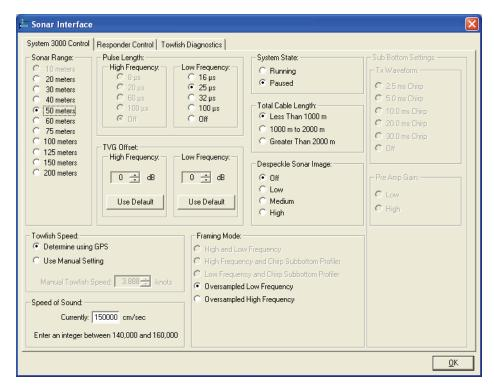
Figure 4-98: The Sonar Interface Dialog Box, Series 3900 Sonar System—System 3000 Control Tab
