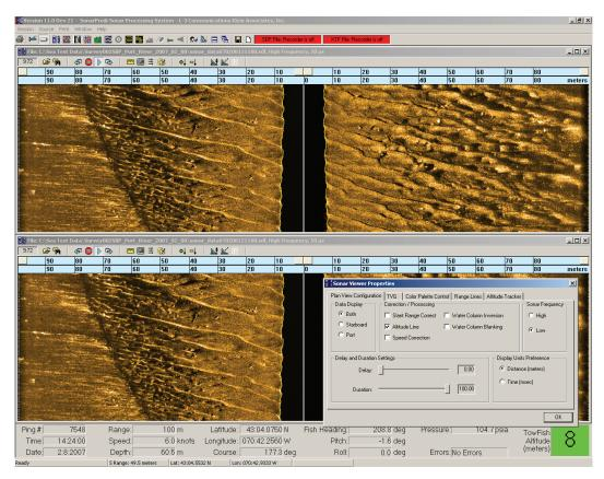
**Figure 4-83:** Sonar Viewer Window—Dual Frequency Operation with the Series 3000 Sonar System
