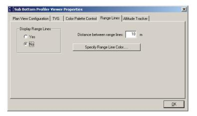
**Figure 4-90:** The Sub Bottom Profiler Viewer Properties Dialog Box—Range Lines Tab
