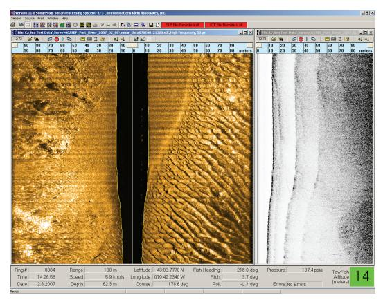
**Figure 4-84:** Sonar and Sub Bottom Viewer Windows—Simultaneous High Frequency Sonar and Chirp Sub Bottom Operation with the Series 3000 Sonar System
