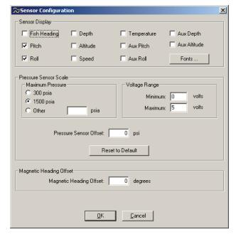
**Figure 4-61:** *The Sensor Configuration Dialog Box*
