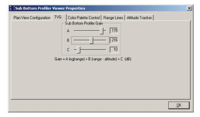
**Figure 4-88:** The Sub Bottom Profiler Viewer Properties Dialog Box—TVG Tab
