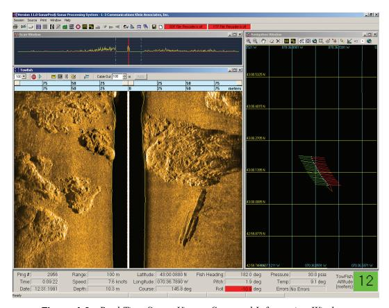
Figure 4-6: Real Time Sonar Viewer, Scan and Information Windows
