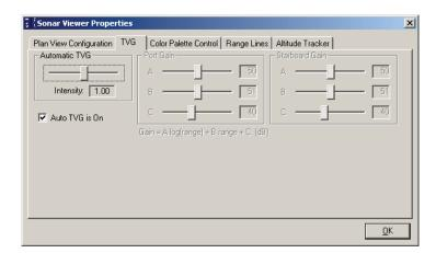
**Figure 4-30:** The Sonar Viewer Properties Dialog Box—TVG Tab
