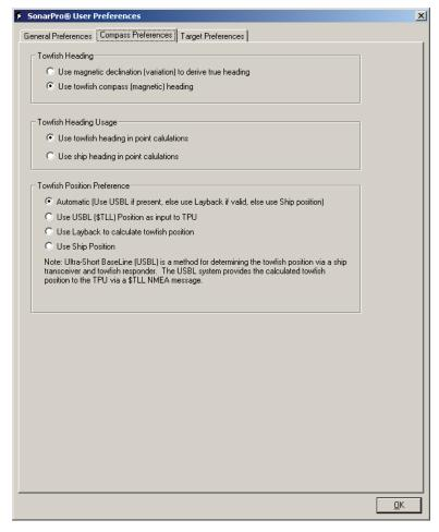
**Figure 4-64:** The SonarPro User Preferences Dialog Box—Compass Preferences Tab
