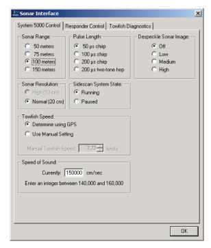
Figure 4-15: The Sonar Interface Dialog Box, Series 5000 Sonar System—System 5000 Control Tab
