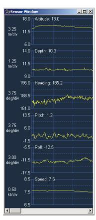
**Figure 4-62:** Example of Sensor Configuration Dialog Box Setup with the Corresponding Results in the Sensor Window
