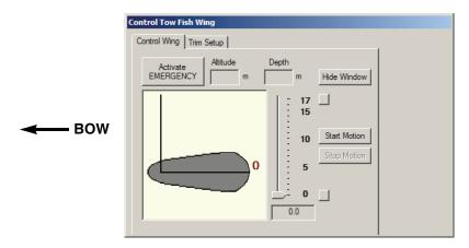
Figure 4-79: The Control Towfish Wing Dialog Box—Control Wing Tab
