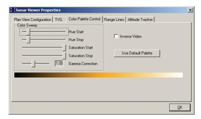
**Figure 4-31:** The Sonar Viewer Properties Dialog Box—Color Palette Control Tab
