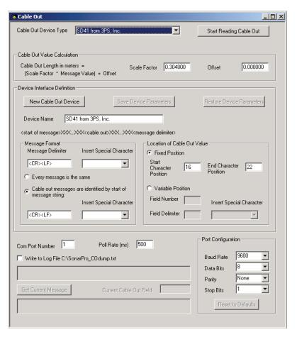
**Figure 4-72:** *The Cable Out Dialog Box*
